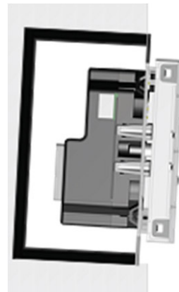
Flush-mounting incorrectly installed
