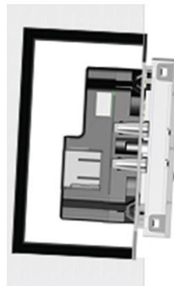
Flush-mounting incorrectly installed
