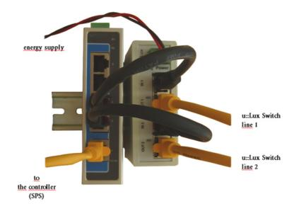
If you use more than 2 *u::Lux NetInj Power* modules, we recommend to wire the supply connections separately to the power supply and not to loop through from one *u::Lux NetInj* to the next one.
