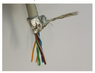
7. Then the individual wires can be sorted and the comb can be mounted. For this example we use the TIA-568B standard.
