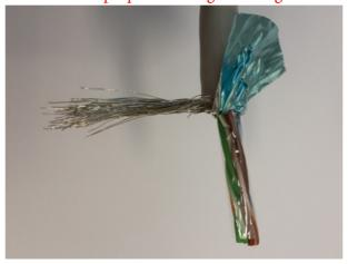
5. Then the plastic foil can be removed. The easiest way to cut off the plastic foil is by using a wire cutter. The foil has no function and would only disturb.
