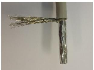
4. Then the foil shielding can be folded back. Attention: The foil shielding must not break off as otherwise a proper shielding can't be guaranteed.
