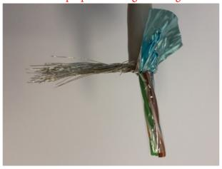
5. Then the plastic foil can be removed. The easiest way to cut off the plastic foil is by using a wire cutter. The foil has no function and would only disturb.
